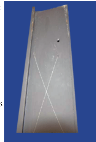
Scribed with 7500 hours Salt Spray- There is no creep from the scribe.
